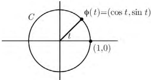
The motion of the particle can be completely described by a function  $\phi : [0, 2\pi] \rightarrow \mathbb{R}^2 : \phi(t) = (\cos t, \sin t)$ .
