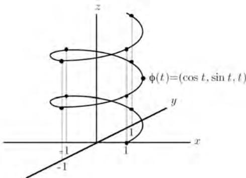
The path has velocity vector  $\phi'(t) = (-\sin t, \cos t, 1)$  and speed  $\|\phi'(t)\| = (\sin^2 t + \cos^2 t + 1^2)^{\frac{1}{2}} = \sqrt{2}$ , so the path has constant speed.
