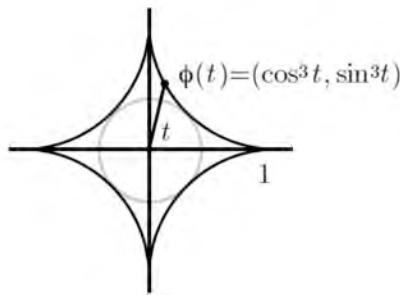
This path has velocity vector  $\phi'(t) = (-3\cos^2 t \sin t, 3\sin^2 t \cos t)$  and speed
