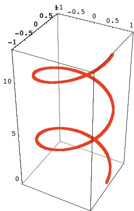
Suppose that  $\phi(t)$  is a differentiable path. We have already indicated that if  $\phi'(t) \neq 0$ , then it is a vector tangent to the path at the point  $\phi(t)$ . We have ...
